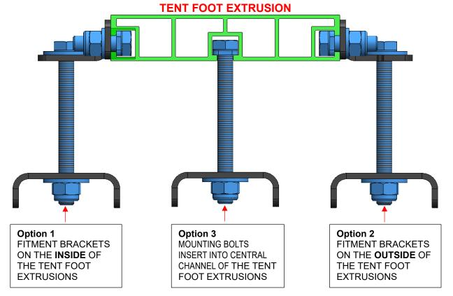
**IMPORTANT**: the supplied nuts and bolts are stainless steel, so it is essential to use an antiseize product on the treads of the bolts (e.g.: Lanotec Type A grease, Nickel Anti-Seize Grease). We also recommend **NOT** to use power tools when tightening the bolts to reduce the risk of seizing an over tightening.
